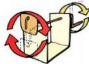
a simple crank mechanism for chewing the head (not shown) is fixed, the lower jaw moves
