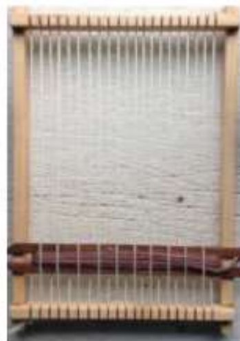
A loom with warp and weft
